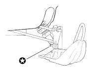
Select feature should be used to achieve the desired ride. The shocks have a wide range of adjustment capability. By turning the screw clockwise, the compression of the shock increases, stiffening the ride. When adjusting these shocks, we recommend that you turn the screw only 1/4 turn at a time, then test ride. Always adjust both shocks equally.
